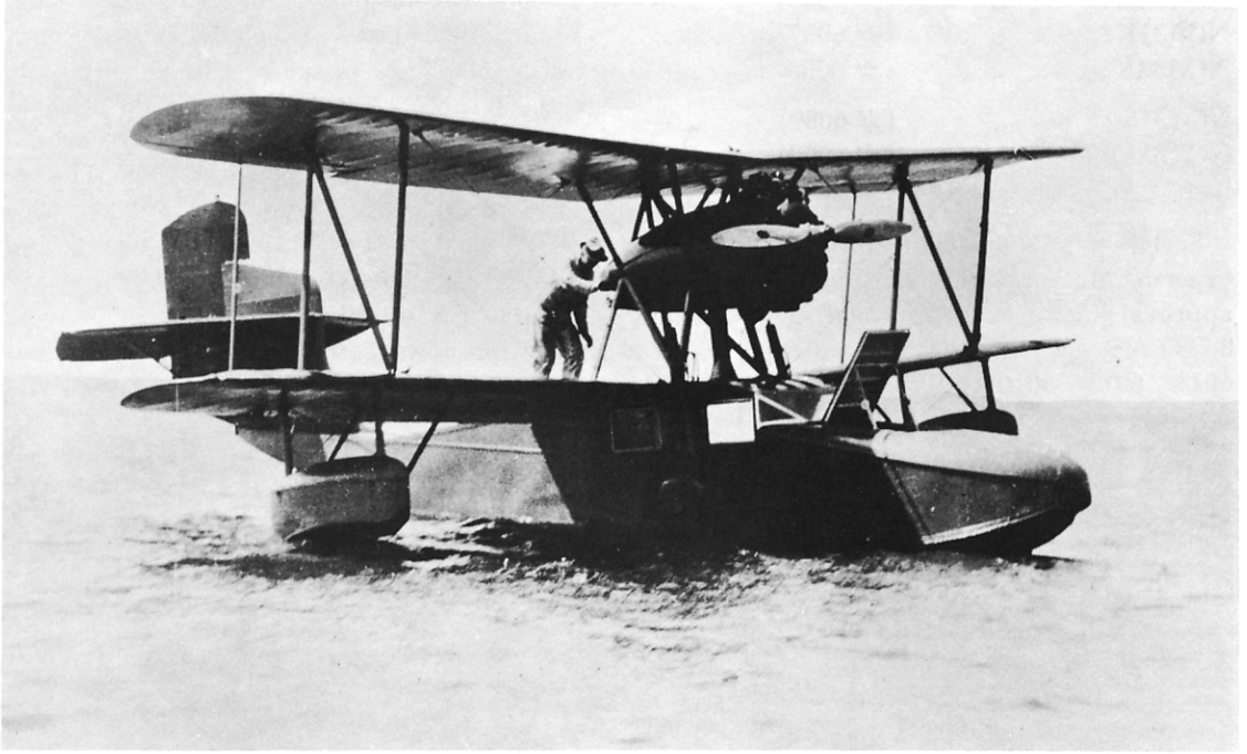
Fig. 61. Keystone-Loening "Commuter" model K-84 with 300 H.P. Wright J6 engine.
