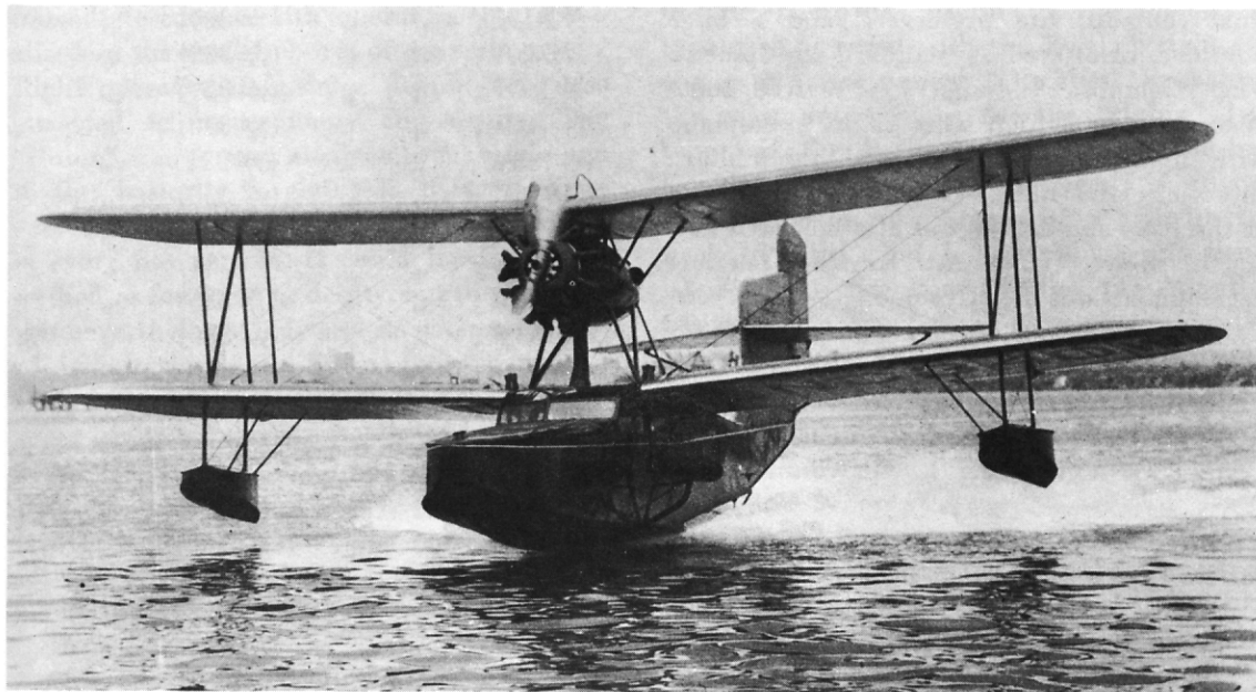
Fig. 62. Commuter behaved well in water; shown here on "step."
