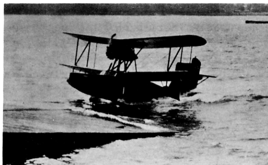
Fig. 64. With gear lowered, commuter taxis up ramp to unload.
