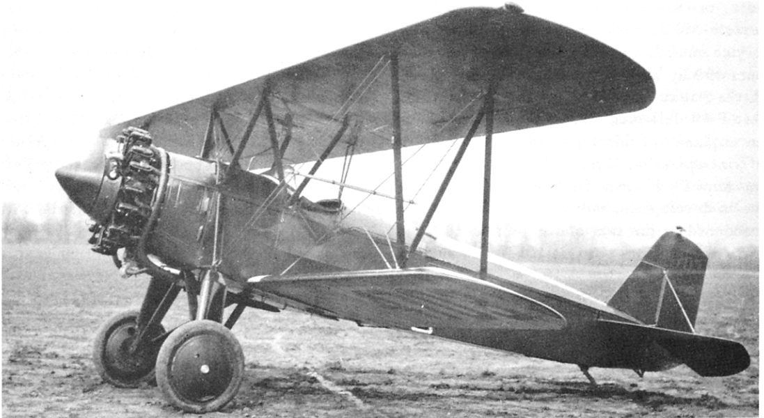
Fig. 182. The 1928 Stearman C3B, powered with "Whirlwind" J5 engine. One of the most versatile airplanes of this period.
