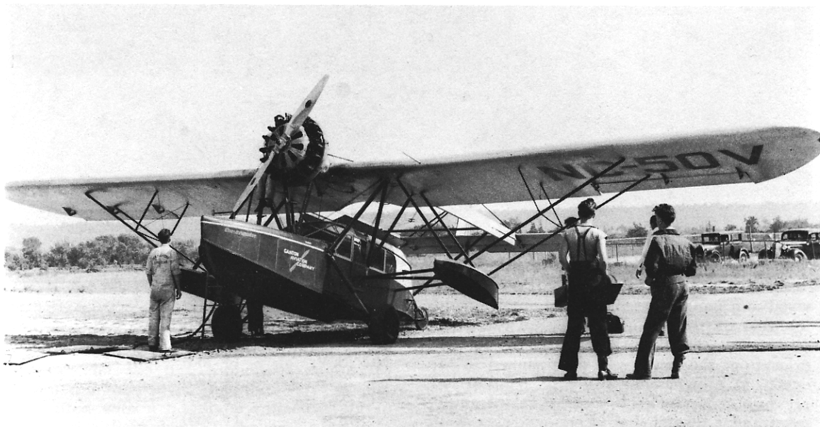
Fig. 231. Improved Sikorsky model S-39-B with 300 h.p. "Wasp Jr." engine.
