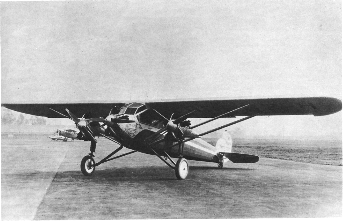
Fig. 74. Kreutzer "Air Coach" model K-5 with 3 Kinner K5 engines.
