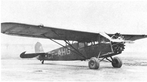
Fig. 206. This FC-2W2 was a long time in Canadian service with Canadian-Colonial Air Lines. Note tail-wheel and Goodyear "air wheels" which were not used in 1928, but were added later.
