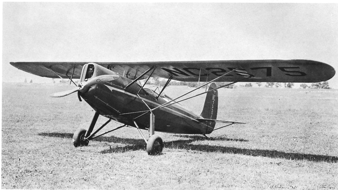
Fig. 8. Fairchild 22-C7D with 4 cyl. Wright "Gipsy" engine. The "Gipsy" and the "Model 22" were a charming combination.
