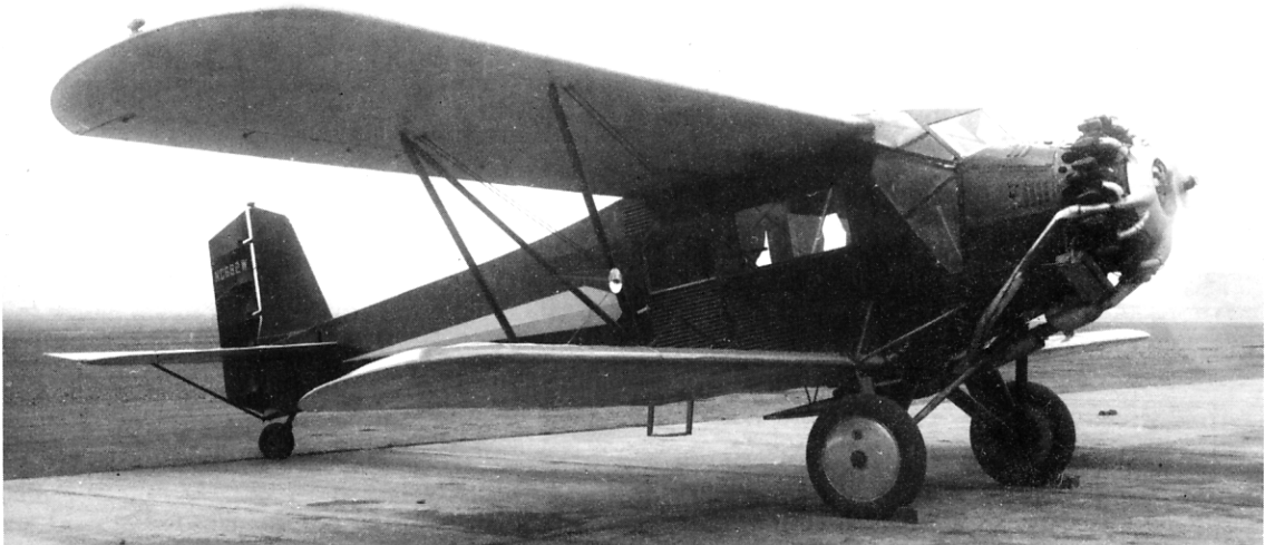
Fig. 248. The PT-6 had a rugged metal structure; its large capacity was ideal for air freight service.
