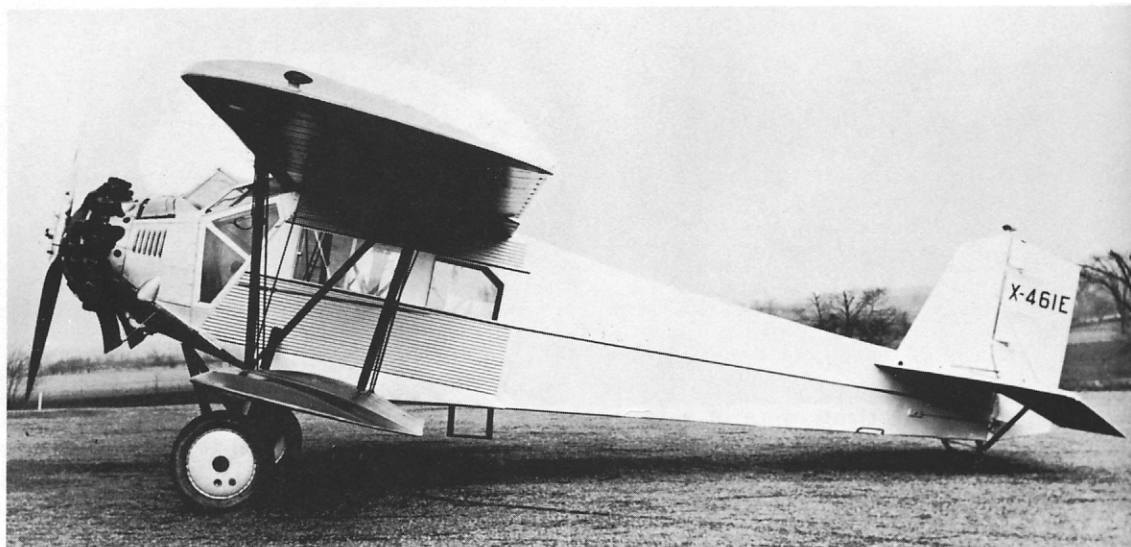
Fig. 247. A Cunningham-Hall PT-6 with a 300 h.p. Wright J6 engine; shown is the prototype.
