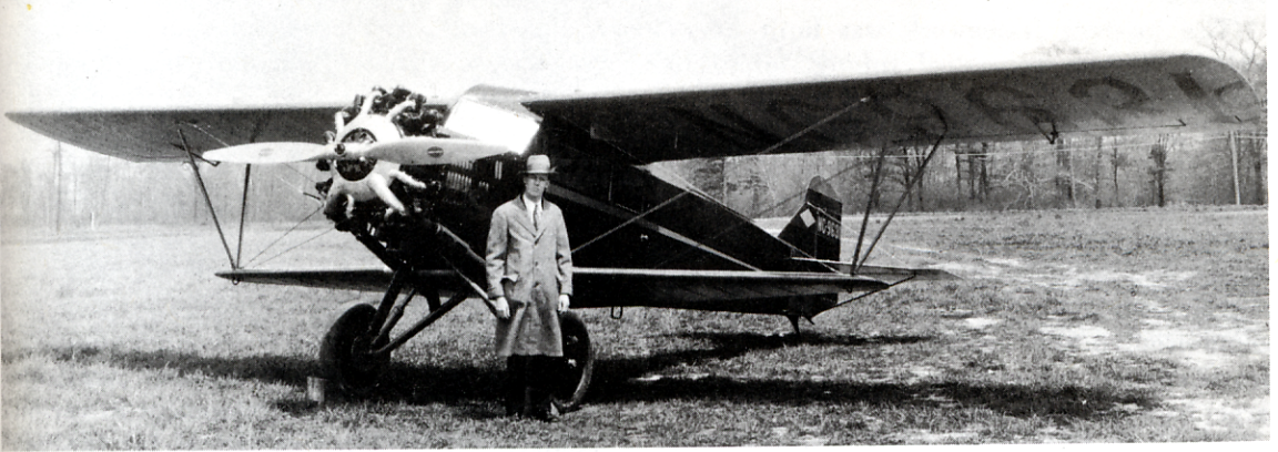
Fig. 205. The Buhl "Sport Airsedan" CA-3D with a 300 h.p. Wright J6 engine.
