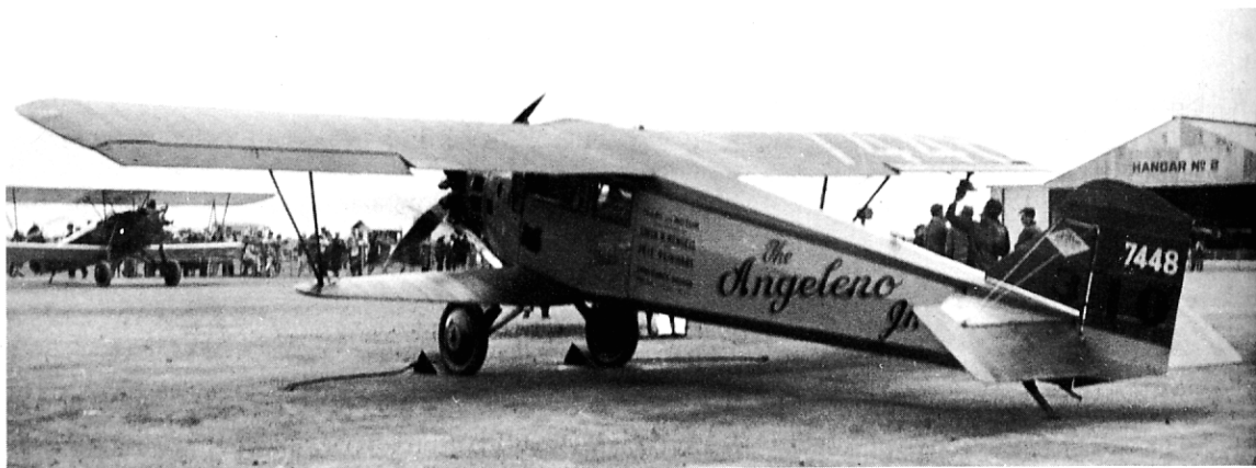
Fig. 206. The "Sport Airedan" was a clean design; note the sesquiplane arrangement.
