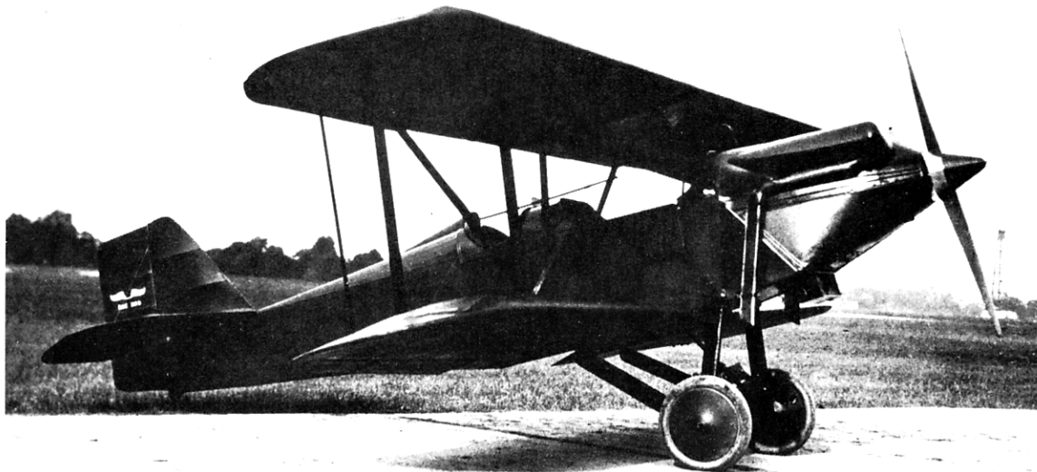
Fig. 252. The "Bluebird" was a Hess design of 1926-27; it was a 3-place craft with the OX-5 or Hisso engine.
